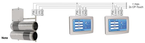
According to the diagram there can be **up four controllers connected to a single unit with RD5 control system**. The last controller connected to the bus bar must have an activated termination resistor – jumper short circuit.
