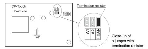
The back of the controller board has jumpers at designated points as shown in Fig. 2 and 3:
